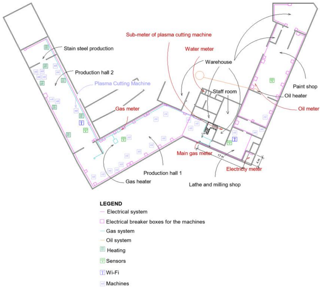
Figure 61: Case Study #3 - Electrical, gas and heating systems as well as sensors location
