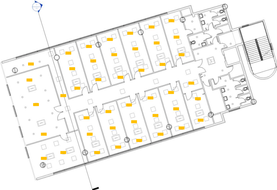
Figure 93: Second floor ground sockets
