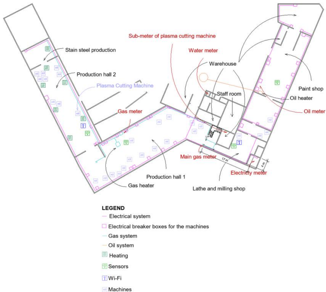
Figure 59: Case Study #3 - Electrical, gas and heating systems as well as sensors location
