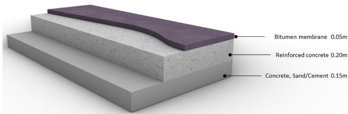
Figure 81: Roof interface from inside out
