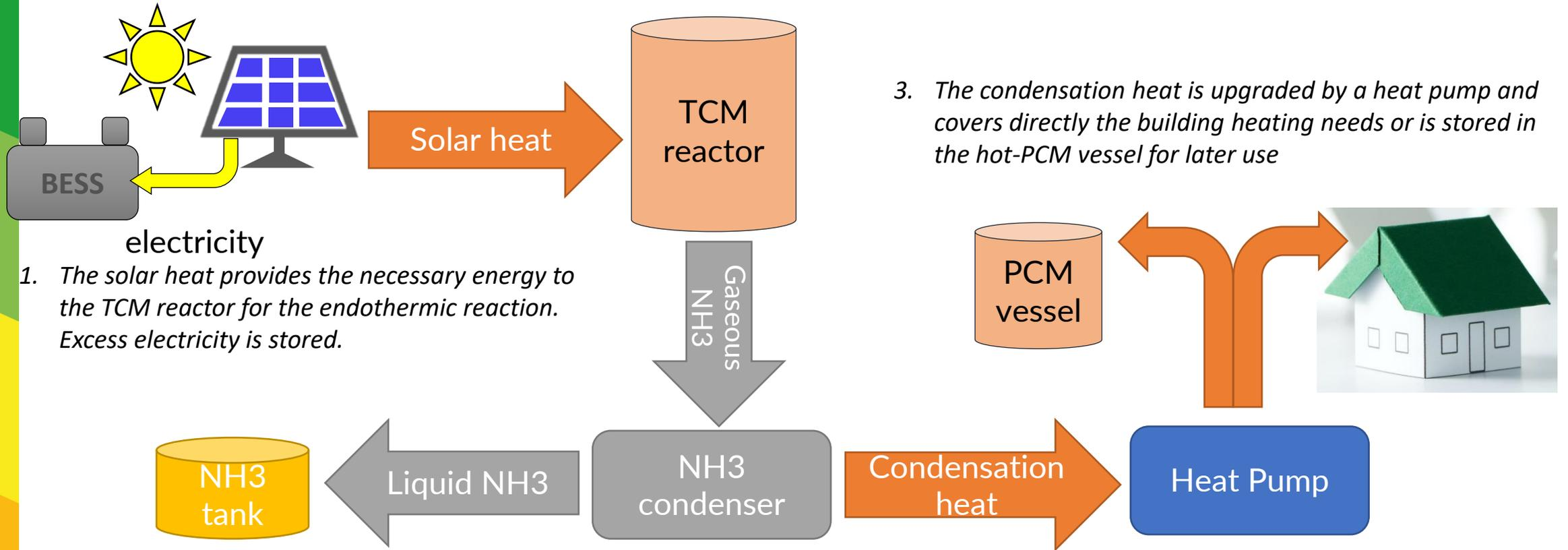
1. The solar heat provides the necessary energy to the TCM reactor for the endothermic reaction. Excess electricity is stored.
